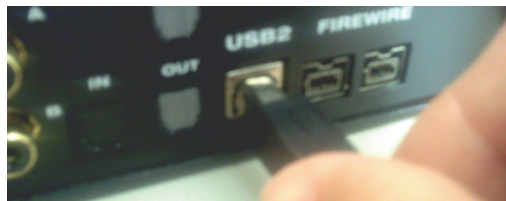
Figure 4-2: Connecting the 896mk3 to the computer via USB.
